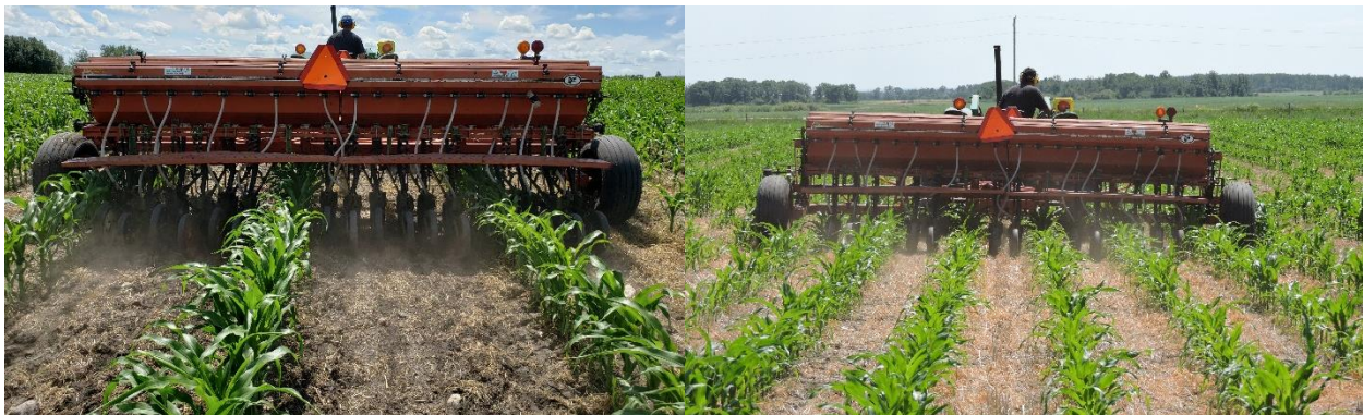
Figure 1. Modified disc drill seeding the corn intercrop. Right: 60" row spacing, July 12 2020. Left: 30" row spacing, July 2 2021. Photos by Jordan Dickson.
